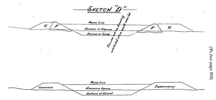
\_\_\_\_\_ Cross Section at Station ——— —<u>240</u>—— \_\_\_\_Scale 30 Feet = linch:—— below the exact grade line of the bottom of the canal works or outside the line of the slopes, unless the same be executed under the written instructions of the engineer.
